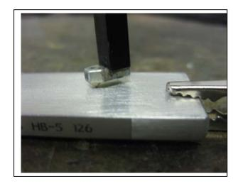
For the existing fleet of over seven hundred Eurostars worldwide, the spar material strength of each aircraft is being spot-checked at the four most critical locations by a combination of hardness and conductivity measurements carried out by Evektor-trained personnel. Of over a hundred sets of wings tested to date throughout Europe, around fifteen percent have had to have the wing spar material replaced because the material was marginally below the minimum acceptable strength figure.
